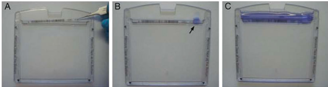
Fig. 3 IPG strip positioning procedure and sealing for the 2-DE second dimension. (a) The IPG strip is placed with the positive end in contact with the left end of the gel; (b) on the right, in contact with the basic end of the IPG strip, is placed a piece of 3 MM for the protein marker loading; (c) strip and markers are sealed with liquid agarose
