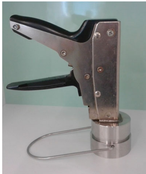
Fig. 1 Appearance of BioPulverizer (BioSpec Products, USA) used for pulverizing knee joints for Real-Time PCR and western blot analysis
