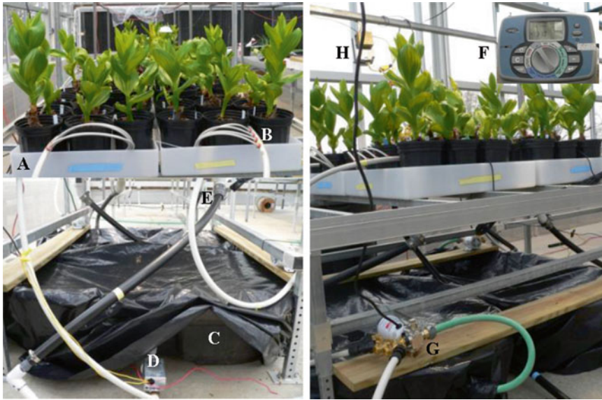
Fig. 4 Overview of ebb and flood sub-irrigation system. Square trays (a) which held either propagative stock plants or micropropagated seedlings. Drip lines (b) dispensed solutions from the stock tank (c) on a regulated basis. The Honeywell motorized valve (d) closes and opens at the drain valve (e) on a timed basis as regulated by the controller (f). The Dayton pump (g) was powered on by the power start relay (h) when the controller sent the signal
