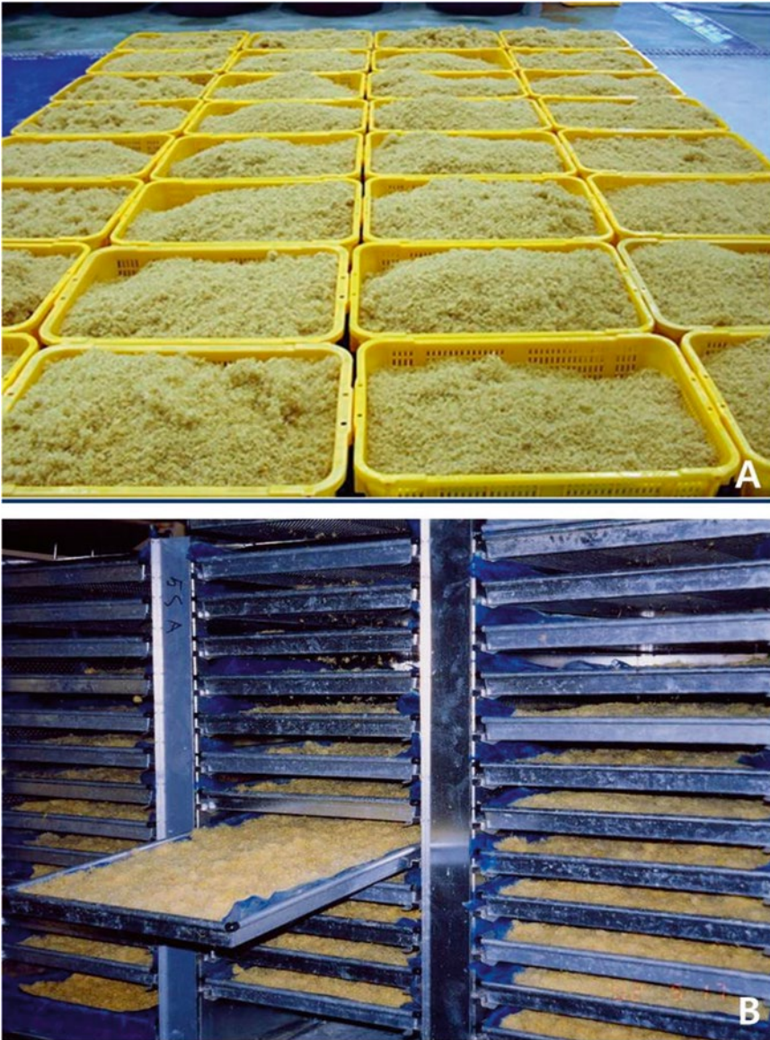
Fig. 5 Ginseng adventitious roots harvested from bioreactors (a), Drying of ginseng adventitious roots in forced air dryer (b)
