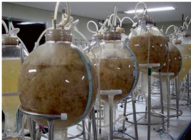
Fig. 2 Adventitious root cultures in 20 L balloon type bubble bioreactors
