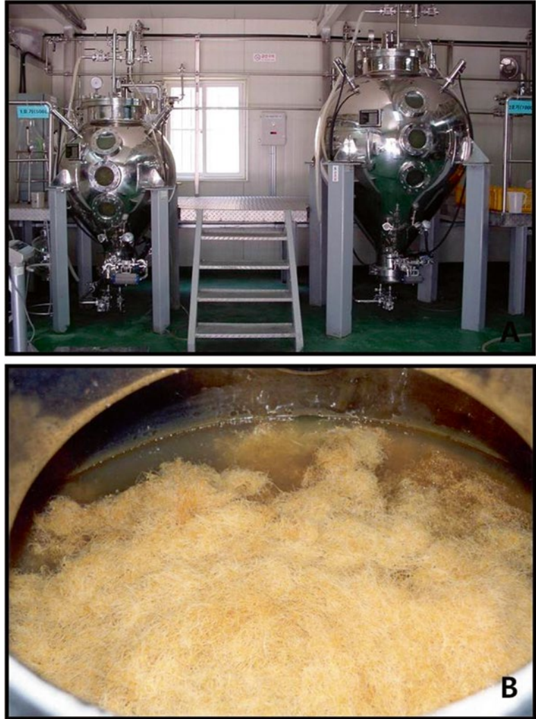
Fig. 3 500 L and 1000 L balloon type commercial bioreactors (a), adventitious root biomass in 1000 L bioreactor (b)
