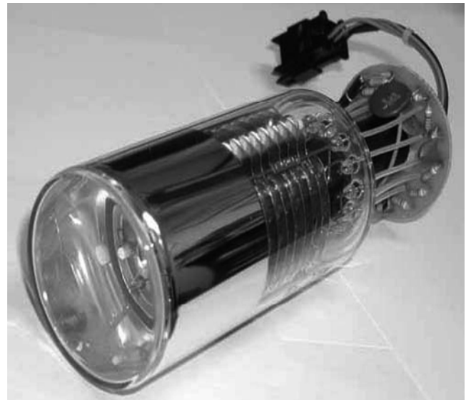
Fig. 11.10 Photomultiplier tube. The left end of the tube is coupled to the crystal. See text for discussion
