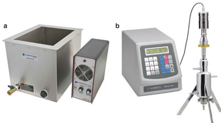
Fig. 11.1 (a) Ultrasonic cleaning bath, and (b) a probe unit
