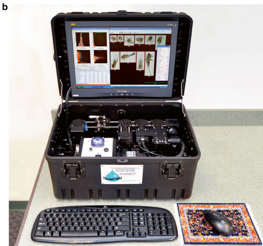
Fig. 1 FlowCam instrumentation. (a) Laboratory benchtop unit. (b) Portable unit
