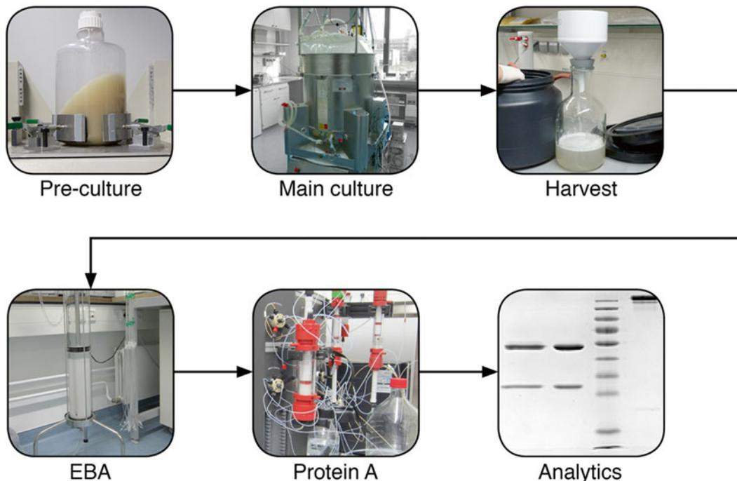
**Fig. 1** Upstream and downstream process steps of 100 L scale antibody manufacture from BY-2 suspension culture. EBA is expanded bed adsorption chromatography; Protein A refers to M12 antibody capture using staphylococcal protein A, which binds IgG molecules by their Fc region
