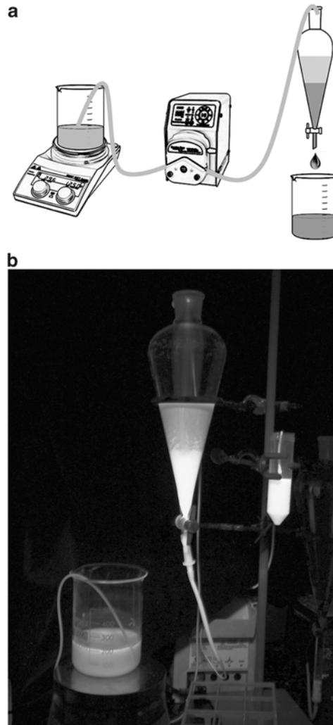
**Fig. 2** Experimental setup for continuous aqueous two-phase separation. (a) Schematic representation of required equipment: magnetic stirrer, peristaltic pump, and separation funnel. (b) Continuous ATPS of GFP-HFBI protein from BY-2 suspension culture extract. The purification setup was imaged under UV illumination
