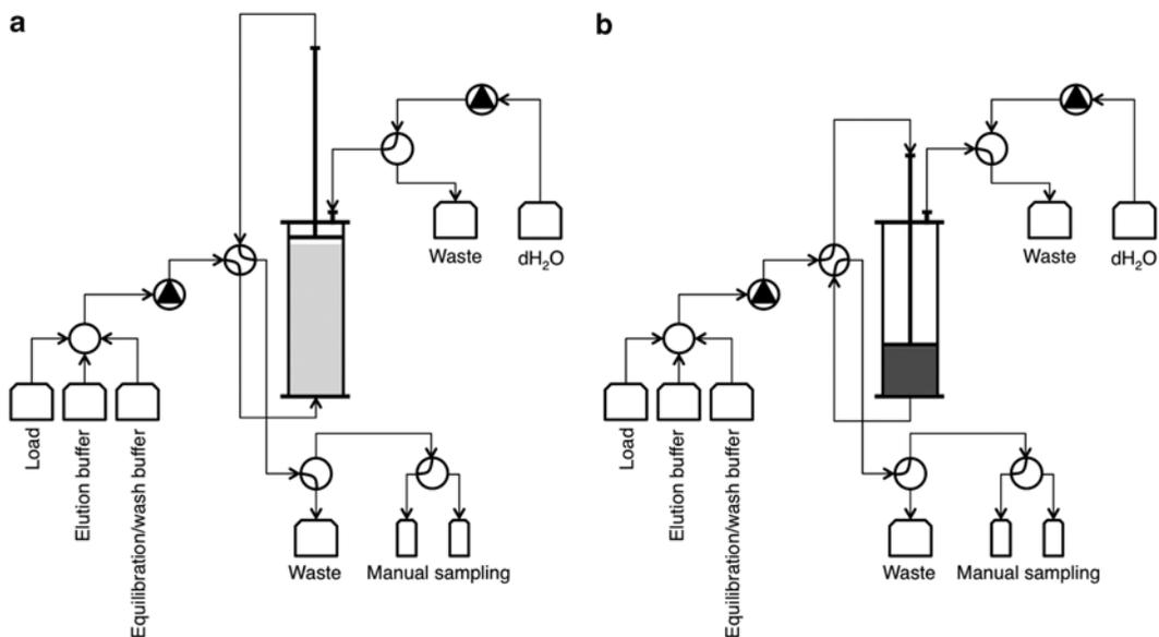
**Fig. 3** Process diagram of expanded bed adsorption (EBA) chromatography: (a) shows the expanded bed mode used during equilibration, sample loading, and washing, (b) shows the packed bed mode used for elution of the antibody
