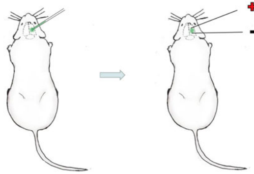
Fig. 3a The schematic diagram of adult electroporation. (a) Adult electroporation using needle like electrode. The nucleic acid solution was injected into the substantial area of adult brain, and the electric pulses were delivered to the target area using needle like electrode. (b) Adult electroporation using tweezer electrode. The electric pulses were delivered to the injected brain in a noninvasive manner, after the nucleic acid solution was injected into the lateral ventricle
