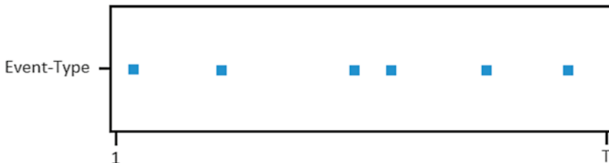
Fig. 4 This figure shows the basic type of data of the T-system, an event-type and its series of occurrence points (unit intervals) on a discrete scale within an observation interval [1, T]
