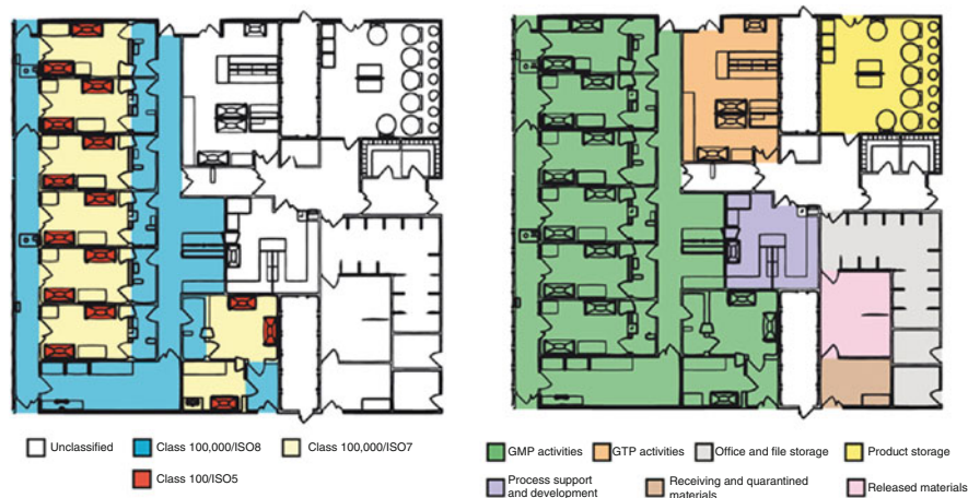
Fig. 7.3 Example of floor plan for clean room production of human cell therapies [105]
