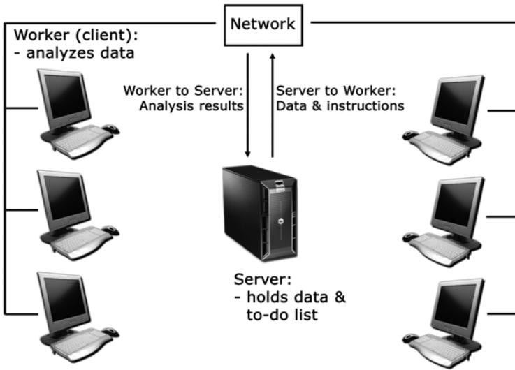
Fig. 8.7 PALAOAdb—a parallel computing system
