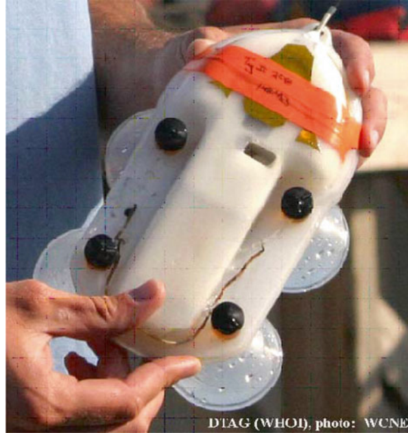
Fig. 1.9 Complete tag including plastic fairing floatation and two suction cups (from Johnson and Tyack 2003)
