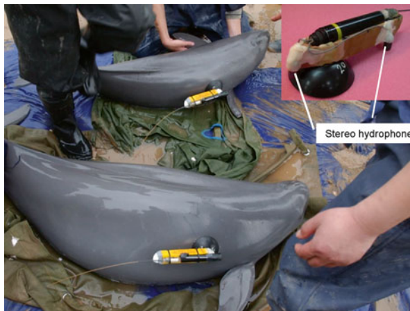
Fig. 14.1 Two finless porpoises ( Neophocaena asiaorientalis ) with A-tag. These animals are ready to be released in a seminatural reserve, an oxbow lake of the Yangtze River in China. The whole system, including an A-tag, a suction cup, and a VHF transmitter were affixed to float material so that it floated after spontaneous detachment from the animal body after approximately 24 h. A VHF radio transmitter with an antenna was used for the retrieval operation. Recorded data in the flash memory of the A-tag were downloaded after the retrieval
