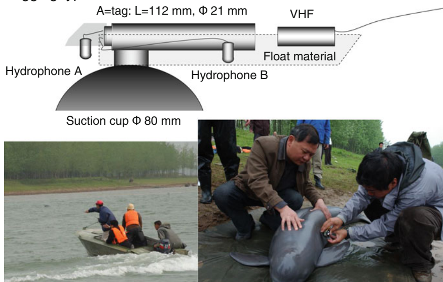
Fig. 14.4 Tagging-type A-tag. After the capture of finless porpoises in the seminatural reserve in China ( left ), an A-tag with a VHF transmitter was carefully attached to the skin on the dorsal side of the animal ( right ). After spontaneous detachment from the animal, the A-tag was retrieved using radio transmission
