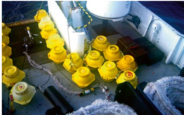
Fig. 6.1 Components of an EARS mooring. These include flotation, the EARS buoys, dual acoustic releases, an anchor chain, and an anchor. Aside from the chain the remaining components are connected by faired cable, to minimize cable strum
