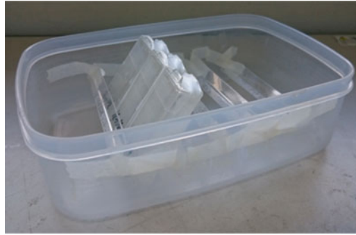
Fig. 3 Setup of coverglass chambers for cultivation. Chambers are placed in a plastic tray at an angle of 80° and incubated in a plant growth chamber
