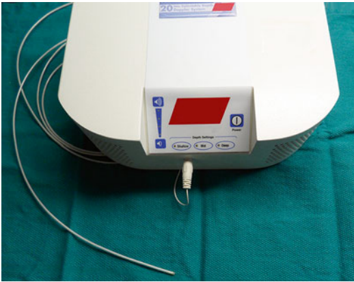
Fig. 6.10 Through-the-scope audible Doppler ultrasound system (processor and disposable through-the-scope ultrasound probe)
