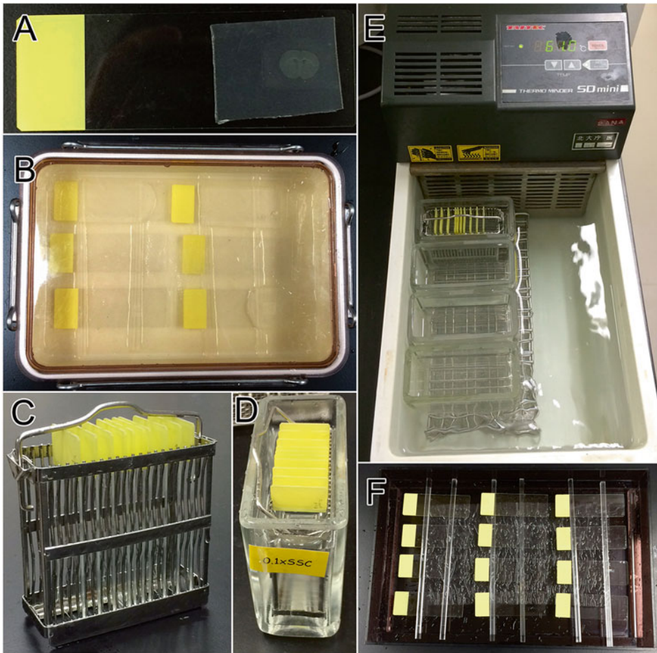
Fig. 1 Key equipment and setup necessary for FISH. (a, b) After applying diluted riboprobes, sections are coverslipped with a sheet of parafilm (a) and placed in a sealed container (b). At the bottom of the container, sheets of filter paper soaked in 50 % (vol/vol) formamide solution diluted with DW are spread to maintain humidity. (c–e) After the overnight hybridization step, parafilm coverslips are removed, and slides are placed in a slide holder (c). Sections are then subjected to a series of post-hybridization washes in conventional glass staining jars (d) that are immersed and preheated in a water bath (e). (f) Blocking and probe visualization through immunohistochemical procedures are carried out in a humid chamber. We generally spread a sheet of paper towel soaked in DW to keep humidity
