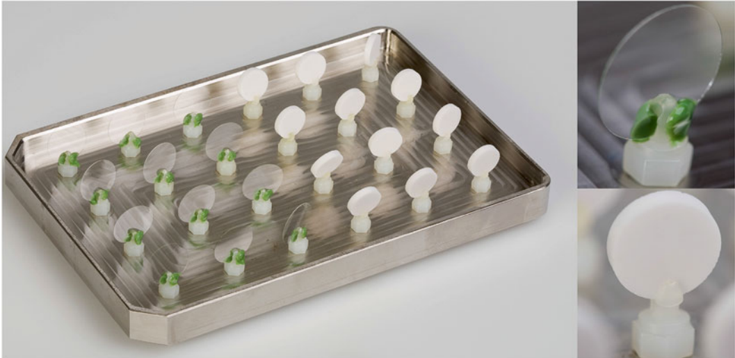
Fig. 1 The AAA model. Left image , a stainless steel lid containing 24 holes to fit pins. Glass coverslips ( top-right ) or HA disks ( bottom right ) can be snap-fixed. Alternatively, thin surfaces might need gluing (President, Coltene, Switzerland)
