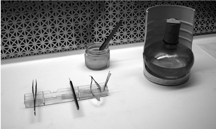
Fig. 1 Typical arrangement of equipment in the clean bench for dissections. The jar in the center contains ethanol and a small layer of cotton in the bottom . The dissecting tools are placed in the jar for at least 10 min, after which the alcohol is ignited by passing the tip over the alcohol lamp's flame ( see Note 9 ). They can then be positioned on a small tray (in this case, it was fashioned from the container in which the microscalpel was purchased) until needed for the dissection
