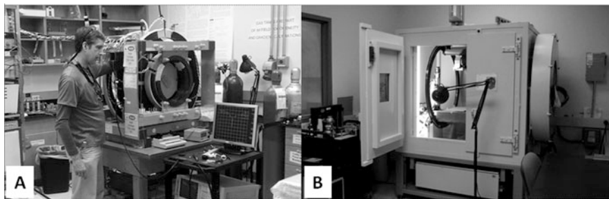
Fig. 23.3 (a) 250 MHz pulse Electron Paramagnetic Resonance oxygen imager. (b) Precision X-ray XRAD225Cx image-guided biologic irradiator/CT imager
