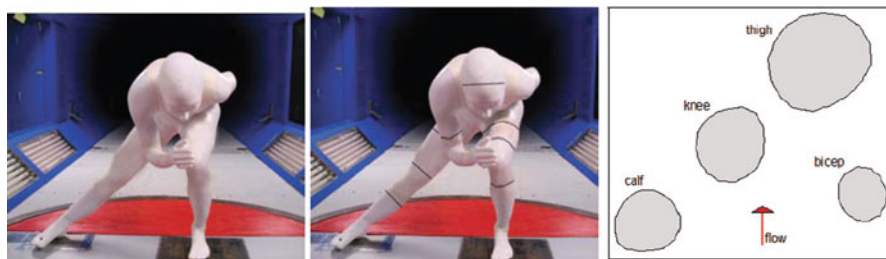
Fig. 8.6 On the left , the mannequin in sidepush position inside the wind tunnel. In the middle , the same model with the locations of pressure taps (the thin circular “lines” one can notice on the mannequin). On the right , cross sections on the right side of mannequin [53]
