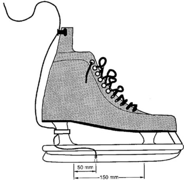
Fig. 3.2 Instrumented skate for direct temperature measurement [14]
