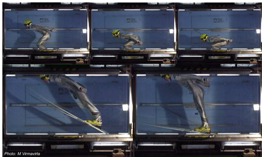
Fig. 6.16 Example of the ski jumping take-off performed with skis in wind tunnel at wind speed of 105 km/h
