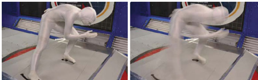
Fig. 8.7 Mannequin in static position at 0^\circ yaw ( left ) and rotating thanks to a turntable from \pm 20^\circ ( right ) [53]
