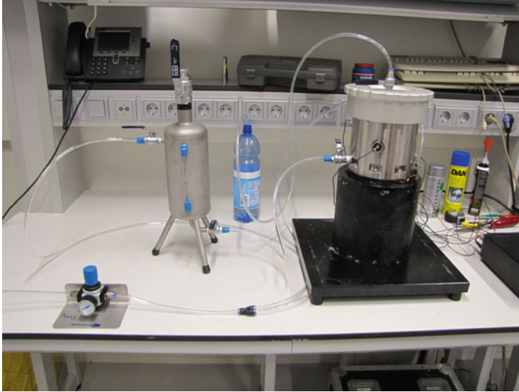
Fig. 11.1 The larvaibrator, a device developed to expose fish larvae to loud impulse sounds. See Bolle et al. (2012) for a schematic drawing of the larvaibrator
