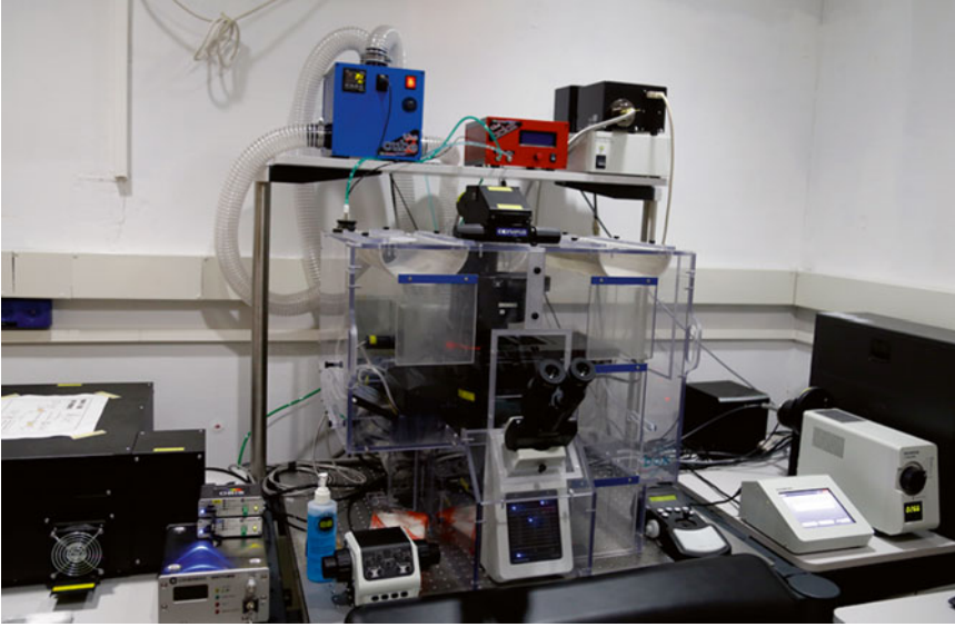
Fig. 4 Commercial microscope temperature-controlled incubator with internal CO 2 incubator (LIS)
