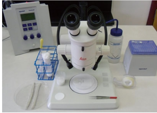
Fig. 1 A prepared work station ready for lining up embryos for microinjection. Upon the desk from the left then proceeding clockwise: needles within their container, a laying chamber tube and a 15 ml tube of Halocarbon Oil with a glass Pasteur pipette ready for covering dessicated embryos, the Eppendorf Femtojet, a water bottle with a fine jet spray nozzle, Eppendorf microloaders (within their tip-rack) and double-sided adhesive tape. Upon the microscope stage (from left to right ) are a small circle of paper for the laying chamber, a recovery beaker, a Whatman paper circle upon a petri dish lid showing a line of embryos ready for transfer, a pair of tweezers and three prepared coverslips
