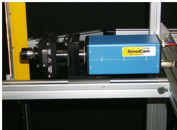
Fig. 6.7 Hyperspectral camera system showing the CCD detector, the housing for the prism-grating-prism spectrograph, and the motor-controlled lens positioning assembly (Lawrence et al. 2003b)
