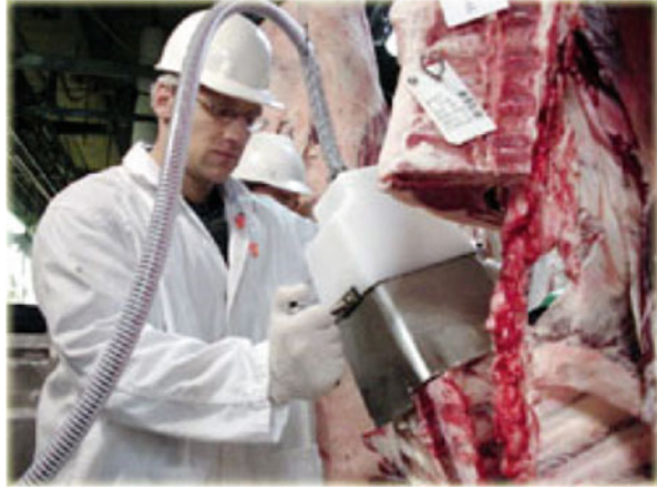
Fig. 10.2 A video image analysis for capturing RGB images of beef ( Source: Research Management Systems, USA Inc., Fort Collins, CO)
