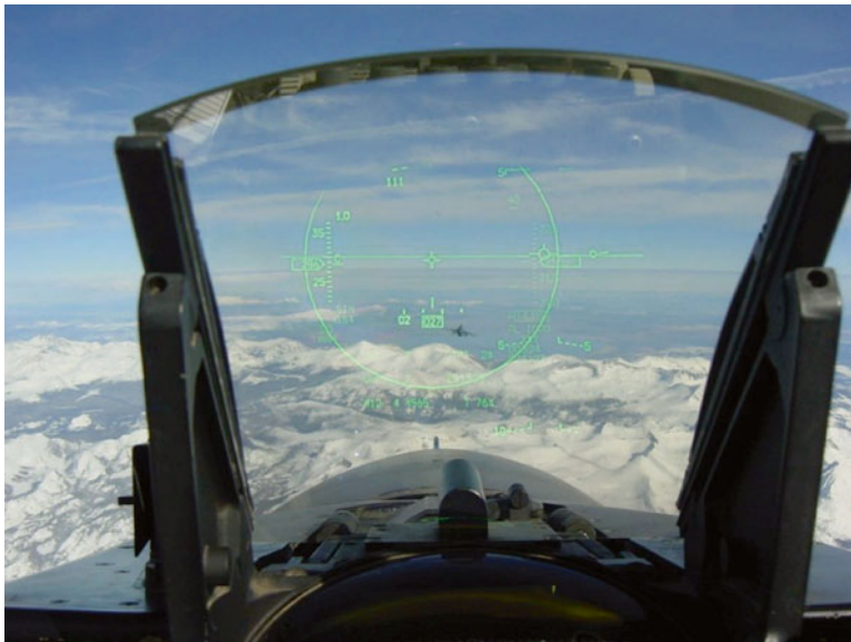
Fig. 6.3 The Heads-Up Display from the cockpit of an F-16 fighter plane displays altitude, artificial horizon, and magnetic heading along with other information to the pilot, without ever losing site of the external environment.
