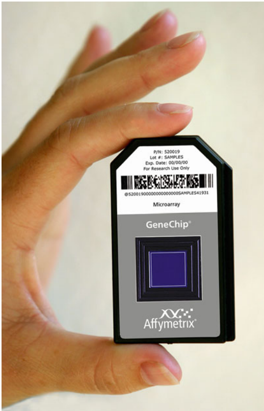
Fig. 3.3 Affymetrix U133 2.0. This is an actual Affymetrix U133 2.0 human GeneChip ® . A single gene chip packed with fragments from each of the 35,000 known genes that make up the human genome. (Courtesy of Affymetrix, Inc., Santa Clara, CA, USA)
