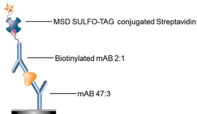
Fig. 1 Schematic illustration of the electrochemiluminescence NfL immunoassay. The carbon ink electrodes are coated with the capture mAB 47:3. The biotinylated detection mAB 2:1 binds to SULFO-TAG labelled streptavidin, which generates electrochemiluminescence signal
