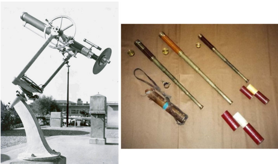
Fig. 5 The original instruments used by R. Wolf. On the left , the standard “4-foot” 80 mm Fraunhofer refractor, pictured here as it was set up at the Zürich Observatory (image source: Library of the ETH Zürich, Image Archive, http://www.e-pics.ethz.ch , Record N° Ans-05063-001). On the right , the three smaller portable refractors (apertures of 30 and 40 mm) used by Wolf while he was travelling
