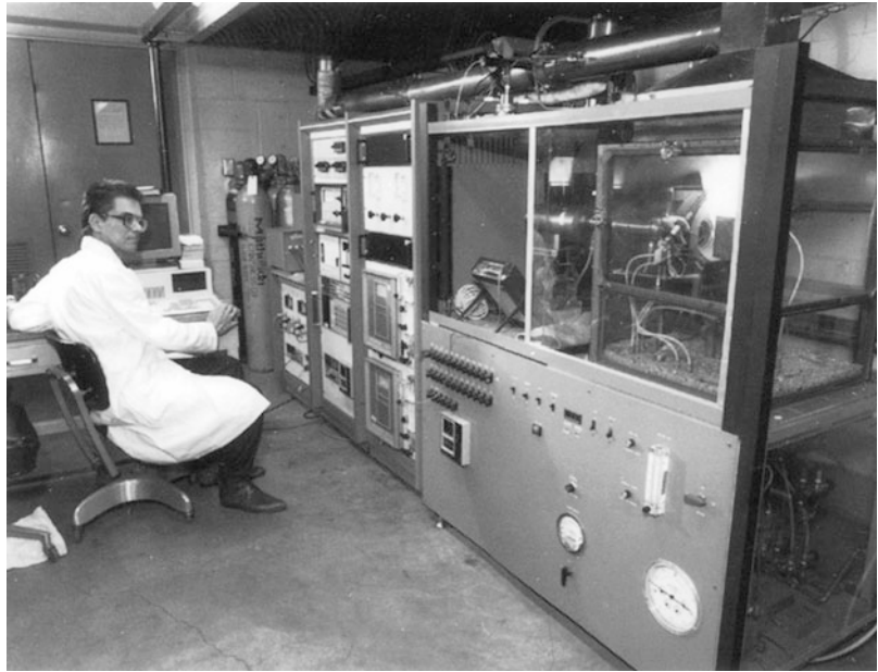
Fig. 28.19 The NIST controlled-atmosphere cone calorimeter
