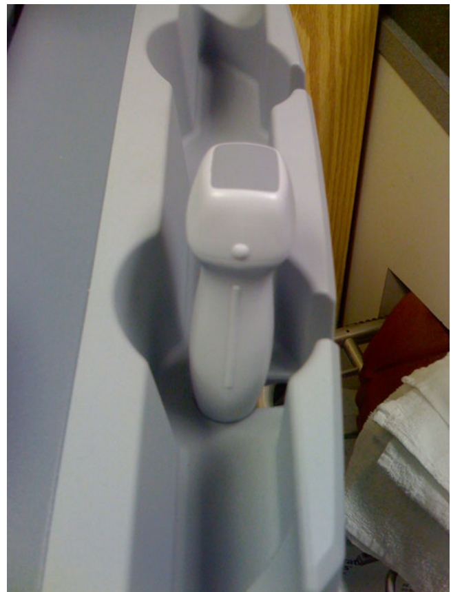
Fig. 71.1 Phased array transducer (P17) with a small footprint that is helpful to fit between the ribs and can be used for focused assessment with sonography for trauma (FAST) examination
