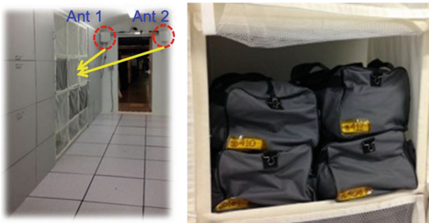
Fig. 18 REALM test bed: RFID Cargo Transfer Bags within a cell of a soft stowage matrix
