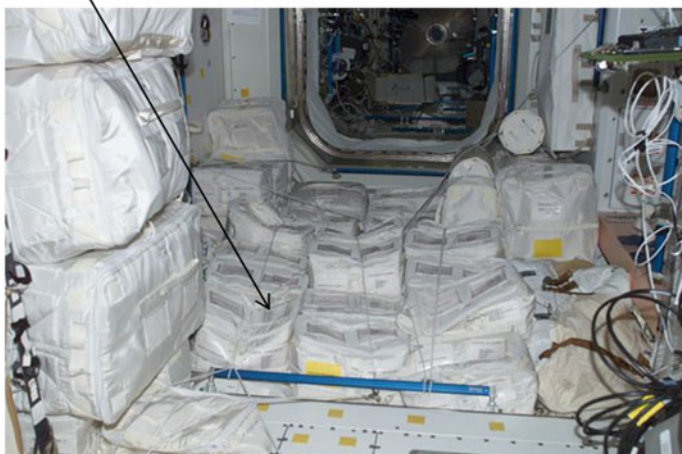
Fig. 13 Cargo Transfer Bags (CTBs) on the International Space Station
