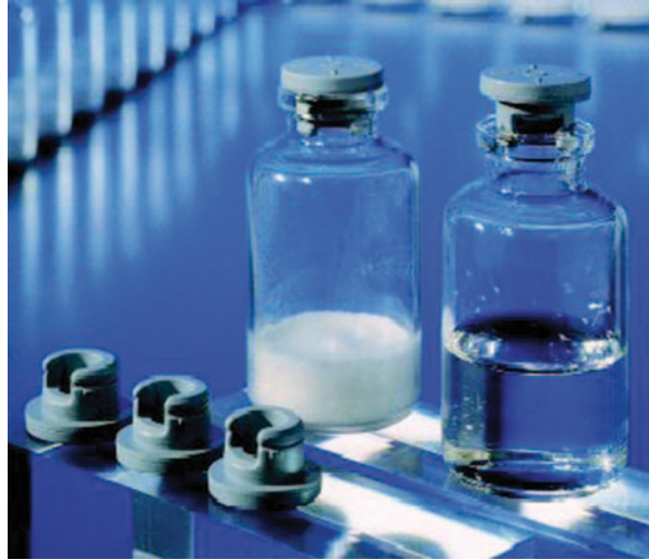
Fig. 1 Half-stoppered vial with drug solution ( right ) and totally stoppered with freeze-drying cake ( left ). In front of the vials: freeze-drying closures with their vent openings facing forward
