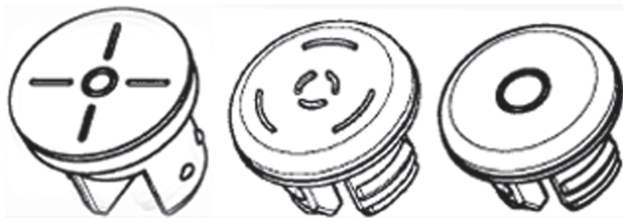
Fig. 2 Lyo stoppers with one, two, and three vent openings, and with different flange markings
