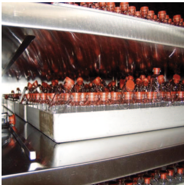
Fig. 3 A shelf of a pilot lyophilization chamber after unsuccessful insertion of the stoppers. Stoppers got stuck to the shelf that pressed them down
