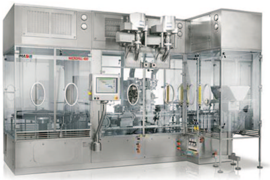
Fig. 6 Sterile powder-filling machine by IMA Pharma ( www.ima-pharma.com ) (Image courtesy of IMA Life North America, Inc.)
