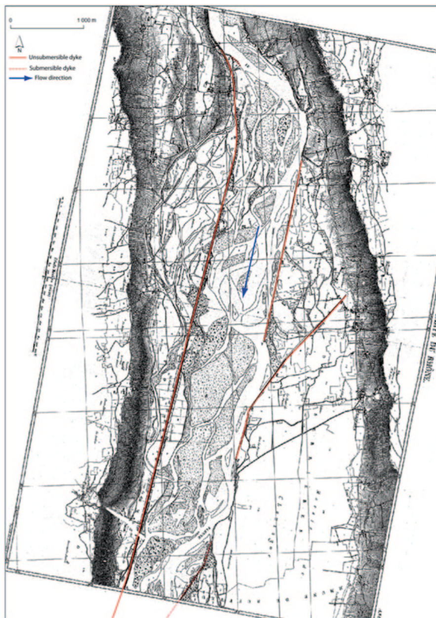
Fig. 9 Location of longitudinal dyke placement to protect land from erosion in Chautagne reach (1860)
