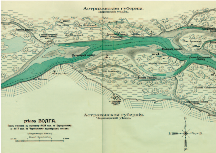
Fig. 13 Zakrutzky section according to a 1914 navigation map. The dashed line is the navigation thalweg. (Source: MPS 1917)
