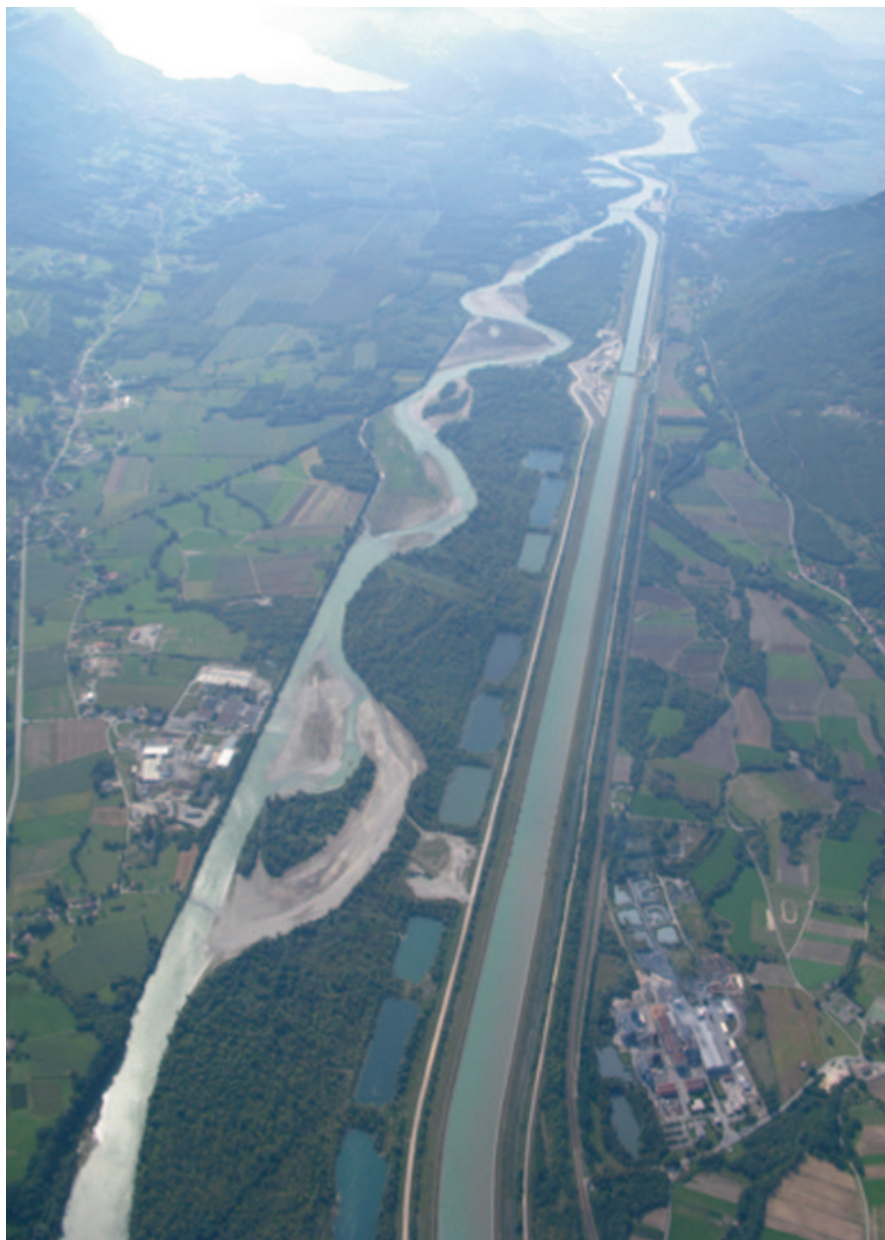
Fig. 10 Photograph of the Chautagne reach seen from upstream. In the north-south Chautagne syncline, the land units are, from the right to the left: the former braided belt, the CNR canal with power plant, the lined gravel pits used to raise the levees of the canal head race, the by-passed Rhône River (“Old Rhône”) with gravel bars and sinuous unique channel, the Chautagne flood plain with former braided belt upstream and marsh (back swamp) downstream. Upper left stands the Bourget Lake. (Courtesy: R. Montagnon/PARACOM/UMR 5600)
