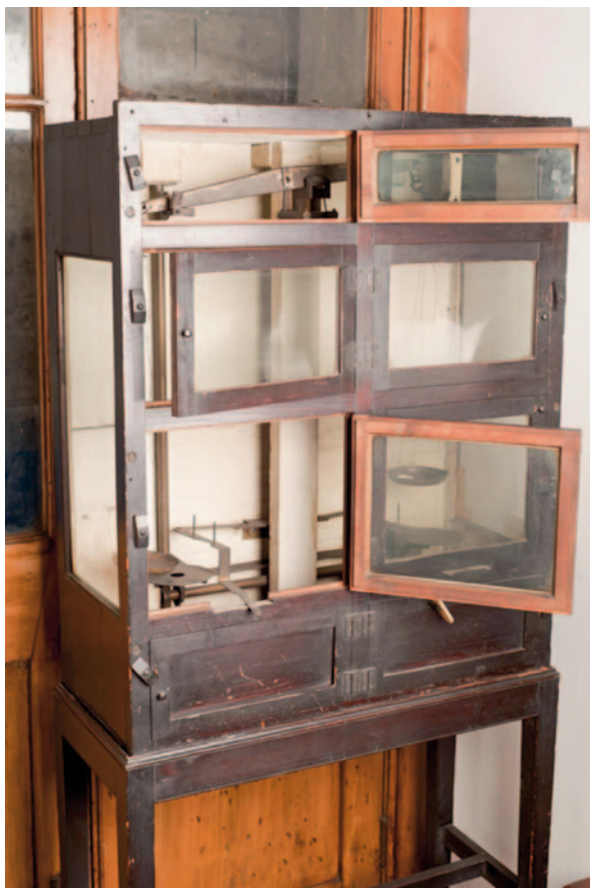
Fig. 13.3 Chemical balance used by Cavendish. This was described as “of rude exterior but singular perfection”. It is now in the Royal Institution in London. (By permission of the Royal Institution)
