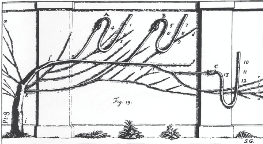
Fig. 8.3 U-tube manometers invented by Hales and used in this instance for measuring pressure developed by sap in a vine
