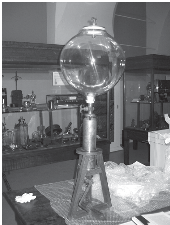
Fig. 4.4 Modern reconstruction of the air pump in the Museum of the History of Science, Oxford, UK. (Reproduced by permission. Photographed by the author)
