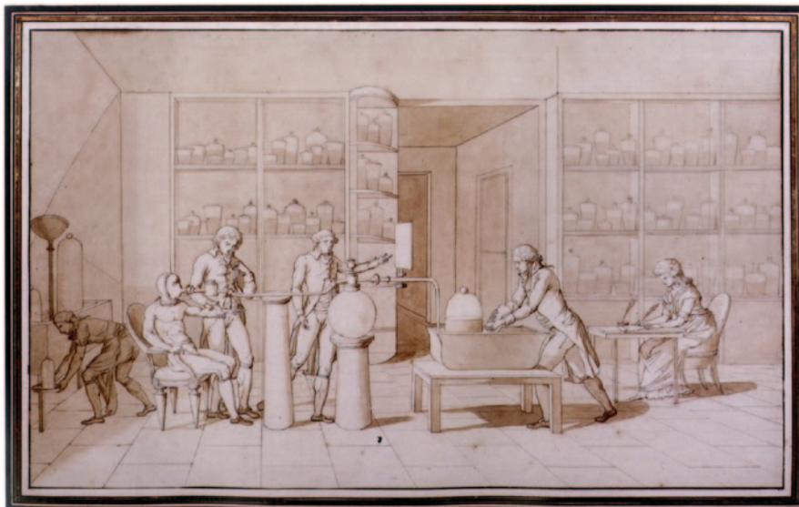
Fig. 12.4 Marie-Anne Lavoisier's drawing of an experiment on oxygen consumption in a resting subject. The expired gas is passed through a glass vessel containing potassium hydroxide in the center and collected on the right by water displacement. Marie-Anne is on the extreme right. See text for details. From [6]
