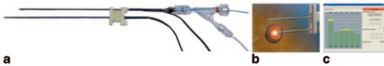
Fig. 19.15 Laser fiber and adjacent thermal probe with the artist's interpretation of the ablation procedure. The
