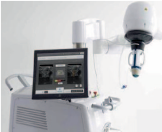
Fig. 19.17 Echopulse, a technology that combines B mode ultrasound with high-frequency ultrasound ablative technology. (Courtesy of Theraclion, Inc.)
