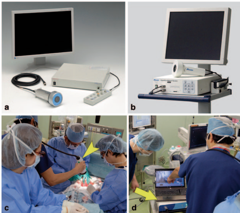
Fig. 22.3 Fluorescence imaging systems for open surgery. a The portable camera head, control units, and TV monitor of PDE®. b Structure of the HyperEye Medical System Handy (Mizuho Ikakogyo Co., Ltd., Tokyo, Japan). c Intraoperative fluorescence imaging with Fluobeam® Imaging System (Fluoptics, Grenoble, France). The arrowhead shows a portable camera head, which can be covered with a sterile drape and used by the operating surgeon. Imaging data is transmitted from a control unit to a laptop PC ( arrow )
