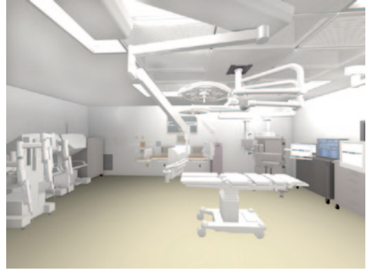
Fig. 1.5 The computer model shows ceiling lights and equipment, OR with data from lighting model to evaluate layouts and sight lines, contrast, and hotspots
