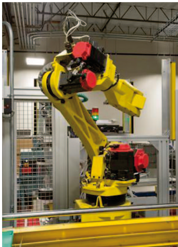
Fig. 20.15 Robotic arm used for automated drop shock testing (Dynamic Automation)
