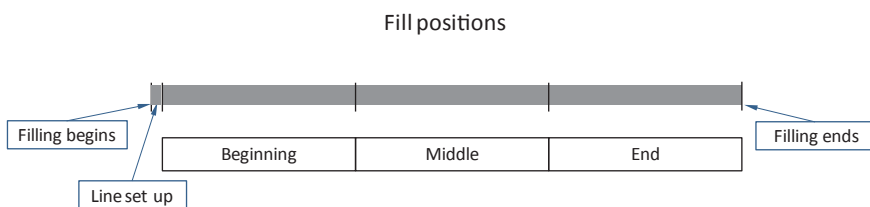
Fig. 26.1 Sampling locations recommended during the filling of a DP batch
