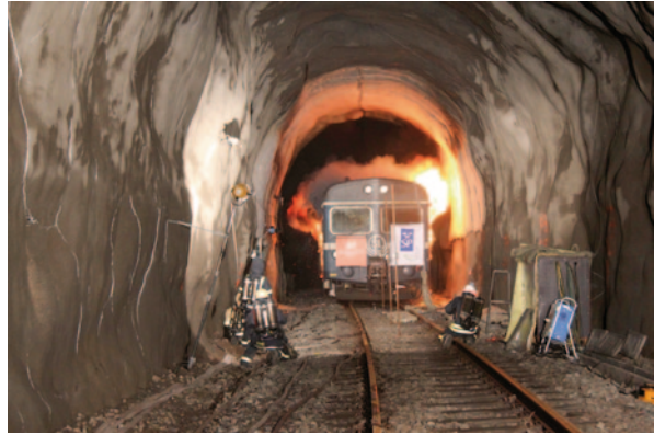
Fig. 1.1 Initial stages of a “flashed over” situation in a metro train carriage. The flames start to plunge out from the broken windows and open doors. (photo Per Rohlén)
