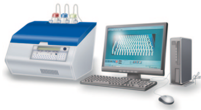
Fig. 10.2 A multitube Autolumat 953 plus luminometer used in the measurement of ROS by chemiluminescence assay. Multiple tubes can be loaded simultaneously for measuring ROS. (Reprinted with permission, Cleveland Clinic Center for Medical Art & Photography © 2011–2013. All rights reserved)
