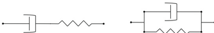
Fig. 1.7 Illustrations of the one-dimensional ( left ) Maxwell and ( right ) Kelvin–Voigt linear viscoelastic models
