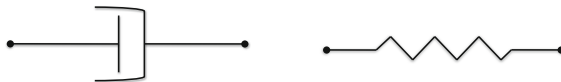
Fig. 1.6 Graphical depiction of two types of material response: ( left ) a dashpot (viscous fluid) and ( right ) a spring (elastic solid)
