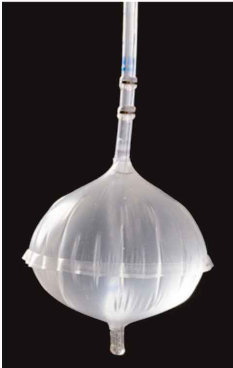
Fig. 5.2 The multimodal probe for electrical, mechanical, cold, warmth, and chemical stimuli. The probe has a bag for mechanical and thermal stimuli, the latter given by recirculating water. Electrodes for electrical stimuli are mounted on the probe above the bag. A side hole in the tube proximal to the bag allows perfusion with acid and other chemicals
