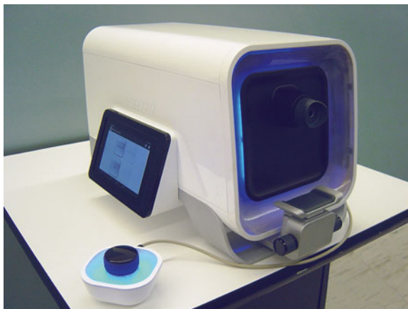
Fig. 10.7 mapcat SF^{\text{TM}} measures macular pigment optical density and lens opacification. Reprinted from [69] with permission from Dr. Karen Thomas
