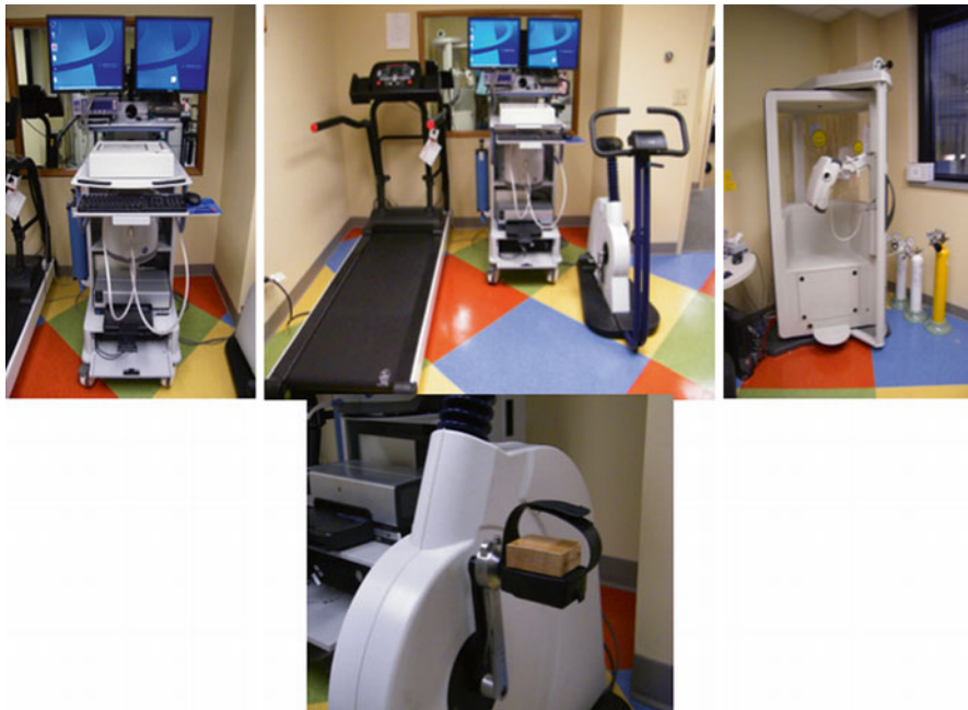
Fig. 12.7 CPET equipment. The treadmill should be long enough to allow runners to reach a comfortable stride length and the side rails must be adjustable for different age groups. The instructions for dyspnea and stopping are posted on the front wall or periodically held up by the technician. The bicycle pedals are adjustable in length as is the seat to accommodate different ages. Blocks can be used if the pedal length does not adjust completely to their leg length. Static pulmonary functions including DLCO should be performed before the CPET preferably on the same day
