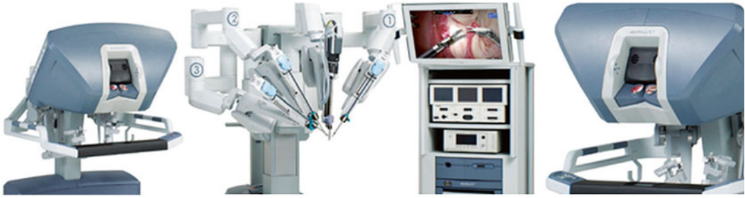
Fig. 1 Schematic demonstrating components of the da Vinci Surgical System, including operator console, Endowrist instruments, and video tower
