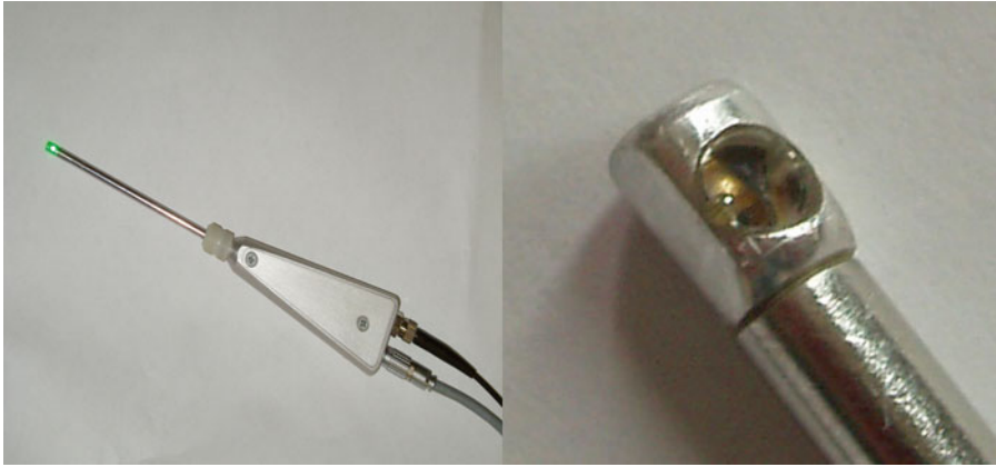
Fig. 14 Optothermomechanical contactor and indenter with two thermocouples [29]
