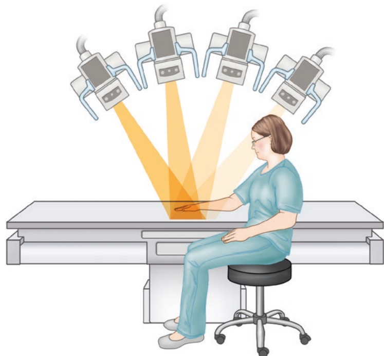
Fig. 1.7 Illustration acquisition tomosynthesis series of hand; note the pathway of the X-ray tube as the images are acquired
