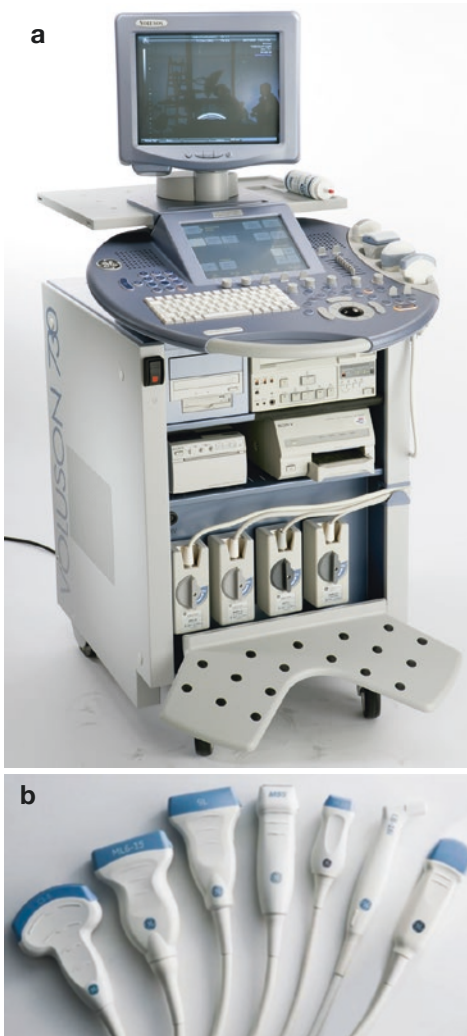
Fig. 1.15 (a) Image ultrasound machine, (b) selection of available transducers for optimization to different body parts
