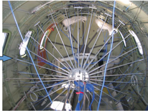
Fig. 5.5 A conformal array of measurement microphones around along the circumference of the interior space of an aircraft while it was cruising at 0.8 Mach number 30,000 ft above the ground. The microphone array was mounted on a track so that it could travel in the longitudinal direction to measure the nearfield acoustic pressure inside the cabin
