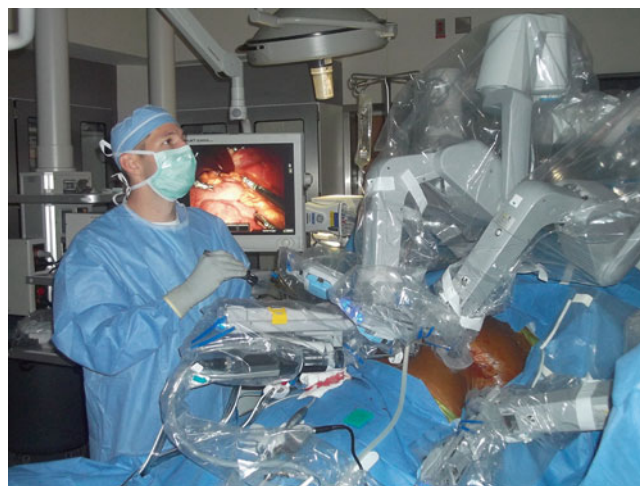
FIG. 23. Robot docked during gastric bypass procedure.
