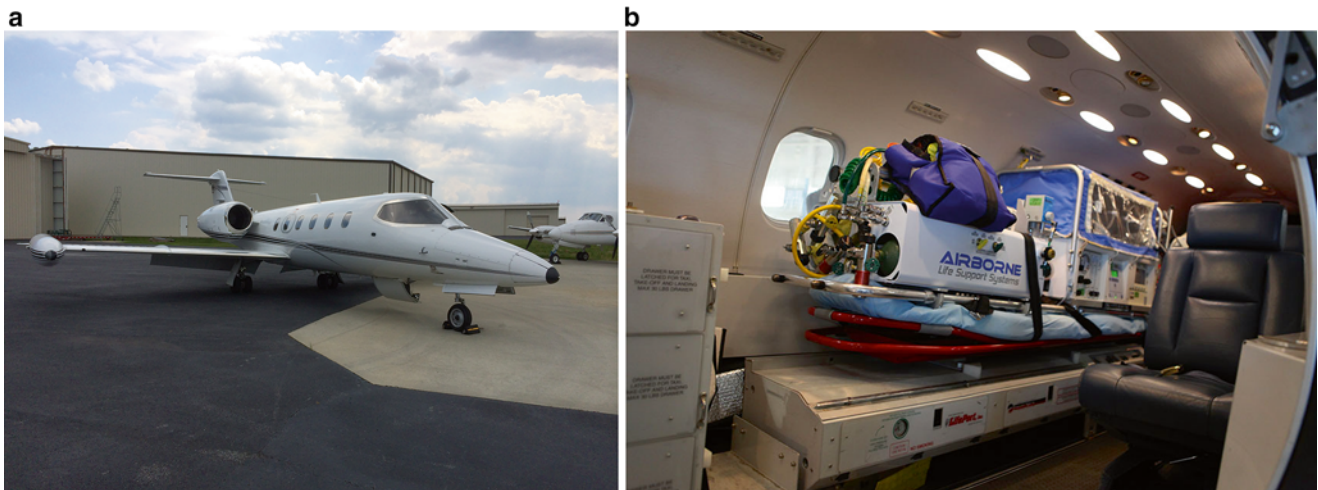
Fig. 12 (a, b) Compact fixed-wing jet used for medical transport with the isolette securely strapped to the anchoring sled
