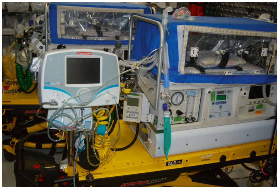
Fig. 3 Neonatal transport isolette with all standard equipment including a “built-in” neonatal ventilator, cardiopulmonary monitoring, inhaled nitric oxide all mounted on a sturdy sled
