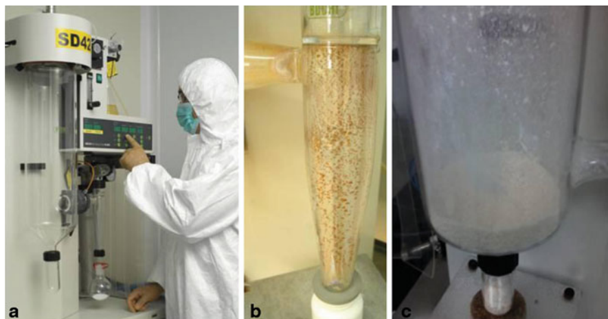
Fig. 8.14 a stable spray drying process, b product degradation in the cyclone, and c bad atomization leading to product accumulation in the bottom of the drying chamber
